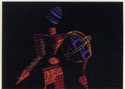
This image of a 3D hierarchical robot has a trackball manipulator attached to its shoulder joint. The arm can be rotated easily by clicking and dragging the mouse on the trackball.
