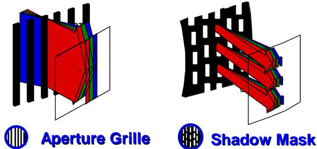
*The all-vertical structure of the Aperture Grille permits more beams to reach the phosphor screen*
