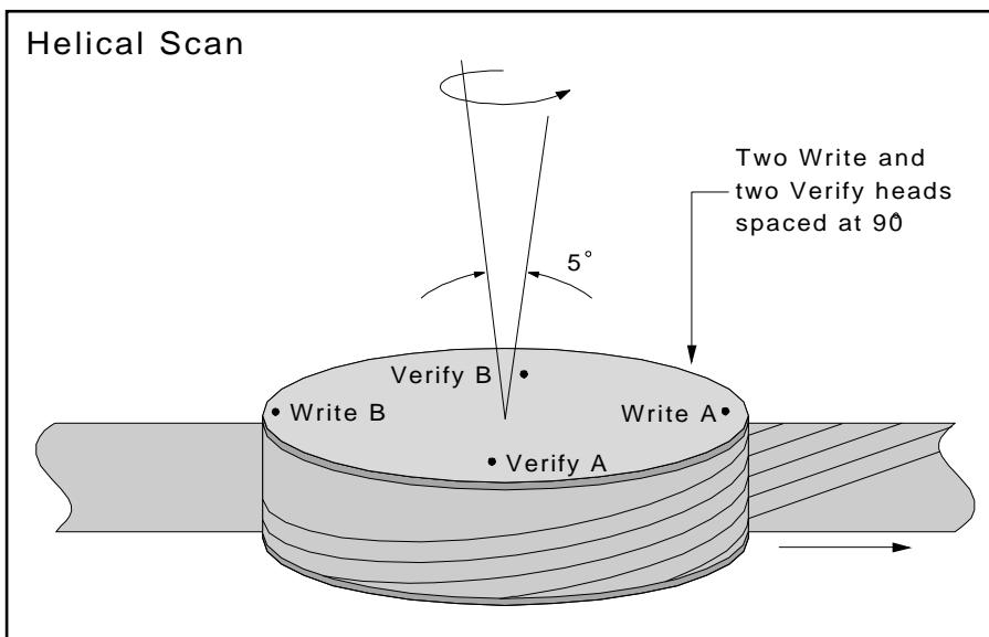
Figure 1. Helical-Scan Heads and Tape with Diagonal Tracks
