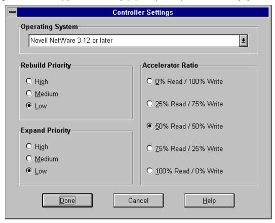
The figure below shows how to enable/disable the Array Accelerator for a particular logical drive. Using the Array Configuration Utility, highlight the appropriate logical volume and use the "Logical Drive/Modify..." option.
