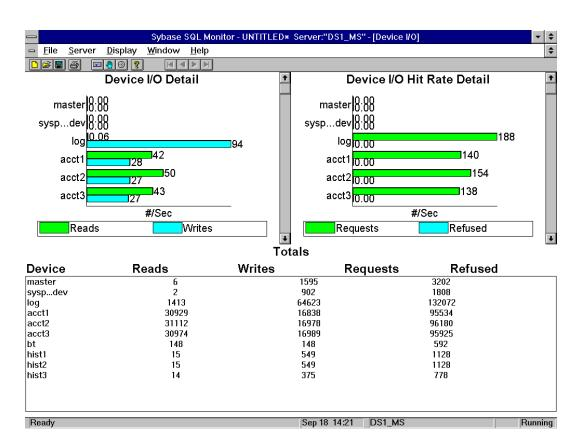
It is best to use values from the SQL Monitor averaged over a period of time to calculate I/O rates. Using the above output as an example, the calculations for determining the number of sequential writes to the transaction log device are relatively simple.
