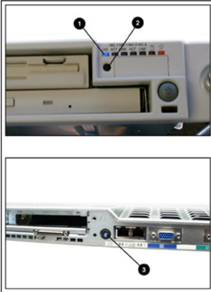
Figure 12: Unit Identification (UID) LEDs and switches on the Compaq ProLiant DL360 server
