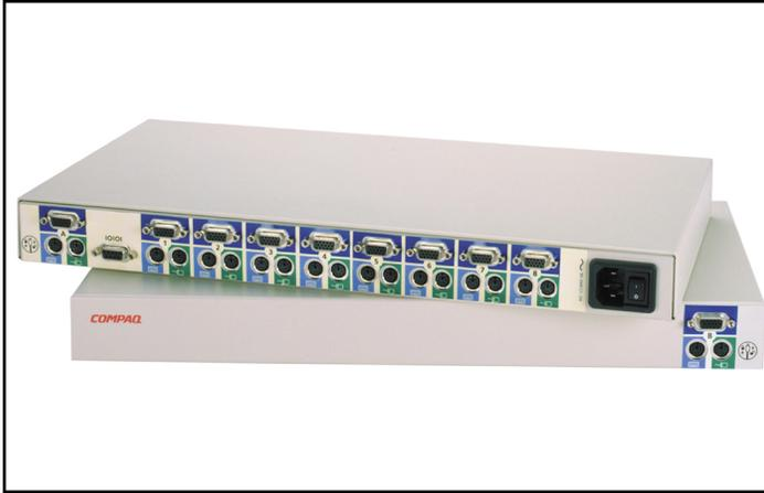
**Figure 16: Server console switches (KVM)**
