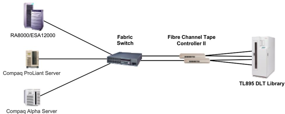
**Figure 1: Enterprise Backup Solution for Legato NetWorker**
