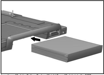
Inserting a Modular Battery Pack or Weight Saver Module into the MCD
