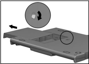
Removing a Modular Battery Pack or Weight Saver Module from the MCD
