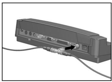
Connecting a Thin-Coaxial BNC Cable to the Convenience Base
