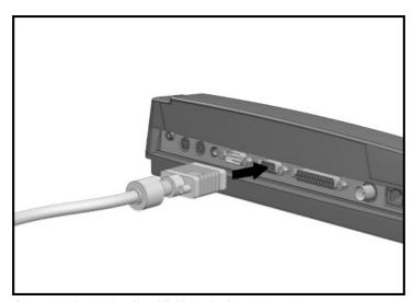
Connecting the Monitor Signal Cable to the Convenience Base
