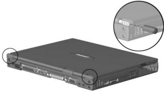
Figure 5-16. Removing the Hinge Covers
