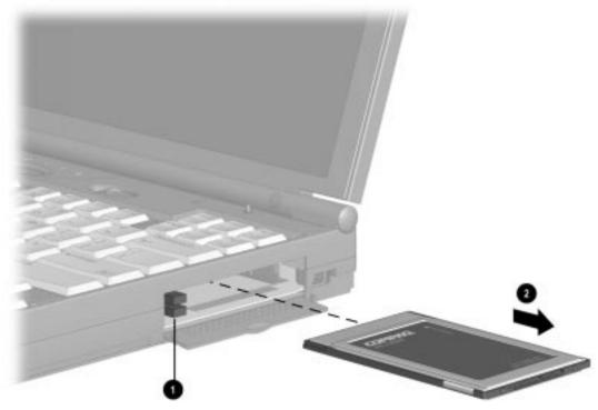
Figure 5-5. Removing the PC Card
