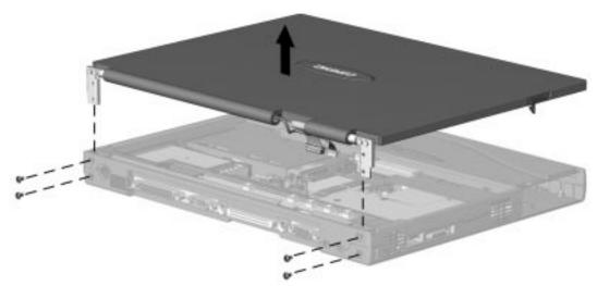
Figure 5-20. Removing the Display Assembly
