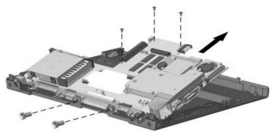
*Figure 5-24. Removing the System Board* To replace the system board, reverse the steps.
