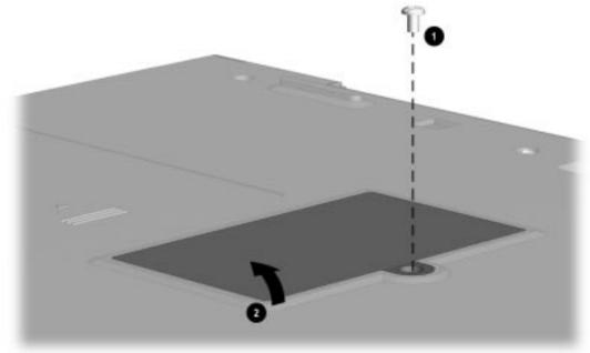
Figure 5-7. Lifting the Memory Compartment Cover
