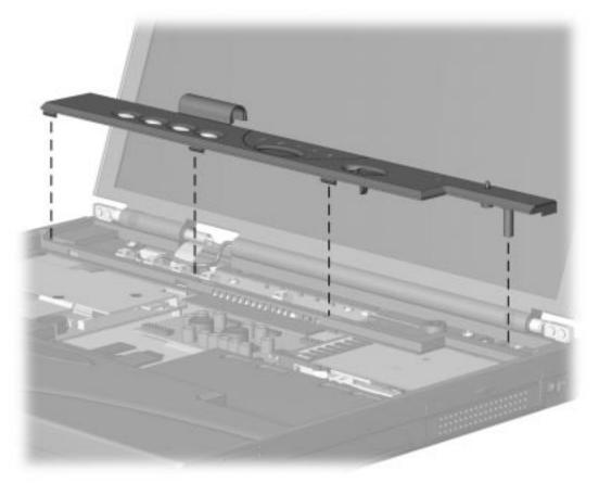
*Figure 5-18. Removing the switch cover/status panel* To replace the switch cover, reverse the procedure above.
