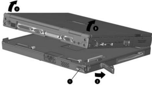
Figure 5-3. Disconnecting the Computer From the Mobile Expansion Unit
