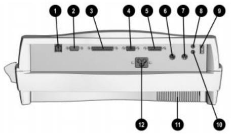
Figure C-3. Convenience Base II with RJ45 Rear Components
