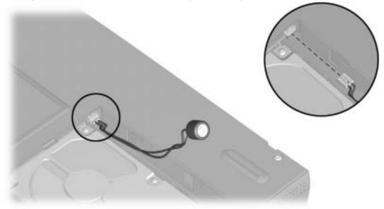
*Figure 5-11. Removing the RTC Battery* Reverse the procedure to install a replacement RTC battery.
