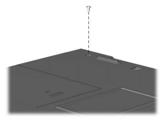
Figure 5-17. Removing the switch cover screw
