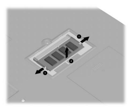
Figure 5-8. Releasing the Memory Expansion Board
