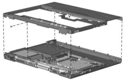
Figure 5-22. Removing the Top Cover Assembly
