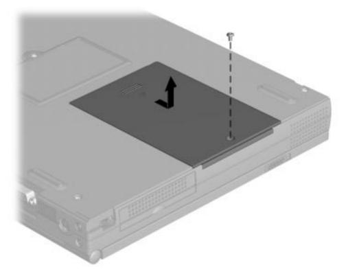
Figure 5-10. Removing the Hard Drive Cover Security Screw
