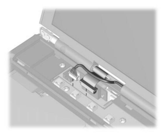
Figure 5-19. Disconnecting the Display Cables
