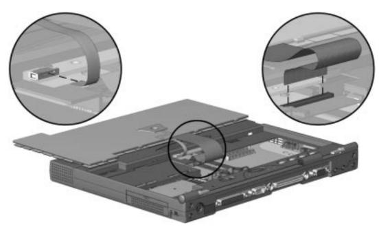
*Figure 5-15. Disconnecting the Keyboard and Pointing Device Cable* To replace the keyboard, reverse the procedure above.
