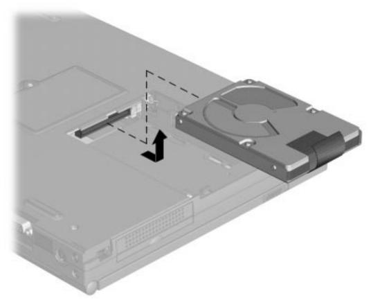
*Figure 5-13. Removing the Hard Drive* Reverse the procedure to re-install the hard drive.
