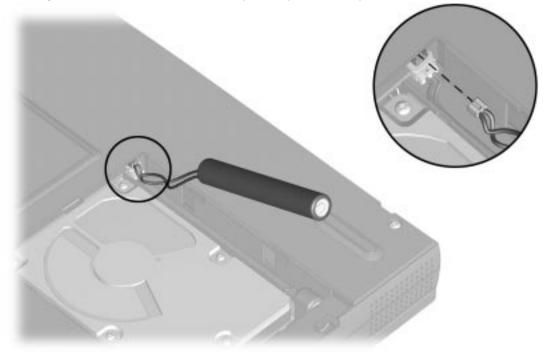
*Figure 5-12. Removing the Standby Battery* Reverse the procedure to install a replacement standby battery.
