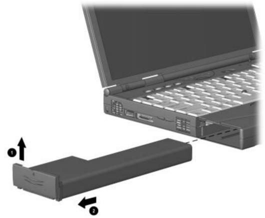
Figure 5-6. Removing the Battery Pack
