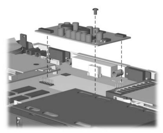
Figure 5-23. Removing the DC-DC Converter
