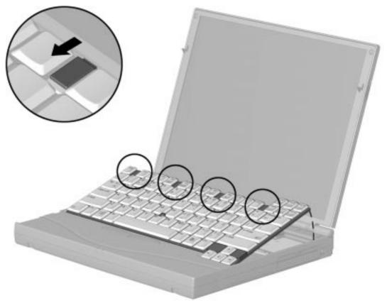
Figure 5-14. Releasing the Keyboard Latches
