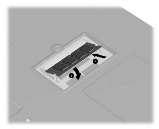
Figure 5-9. Installing the Memory Board
