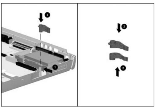
Figure 5-57. Installing the PC Card Eject Levers
