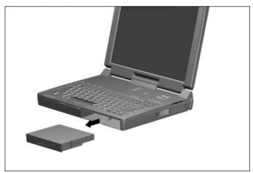
Figure 5-24. Removing a Drive from the MultiBay
