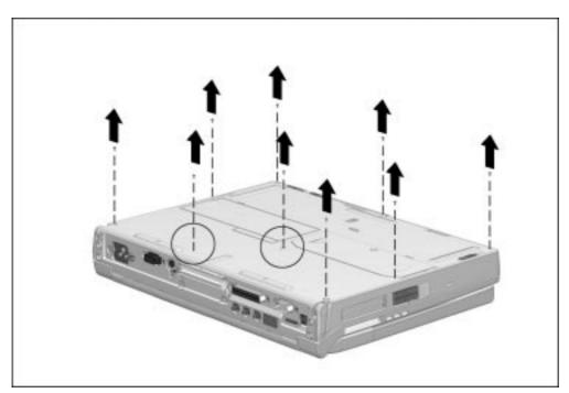
Figure 5-30. Removing the Keyboard Assembly Screws
