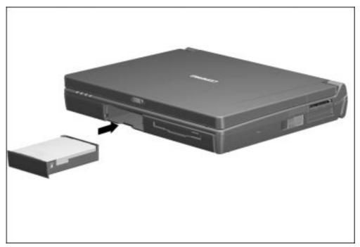
Figure 5-19. Inserting a Hard Drive into the Hard Drive Bay
