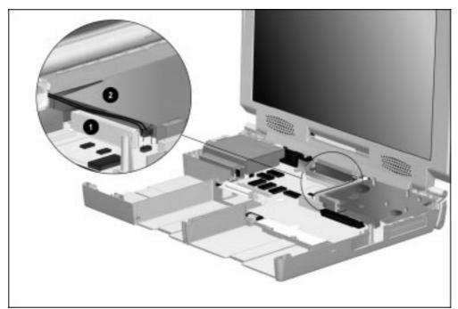
Figure 5-55. Connecting the Auxiliary Battery Cable to the System Board
