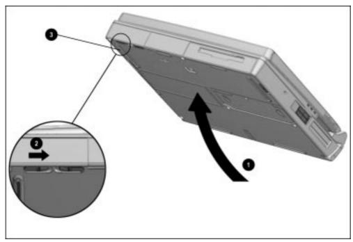
Figure 5-9. Releasing a Battery Pack from the Battery Bay
