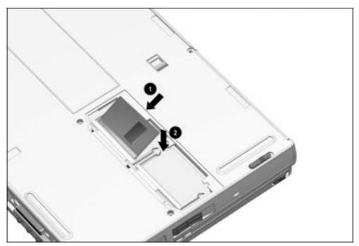
Figure 5-28. inserting a Memory Expansion Board
