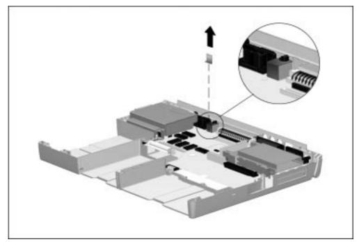
Figure 5-59. Removing the Keyboard Connector Insulator
