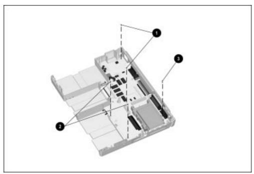
Figure 5-60. Removing the System Board Screws
