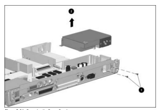
Figure 5-34. Removing the Power Supply
