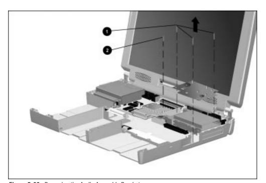
Figure 5-39. Removing the Audio Assembly Bracket
