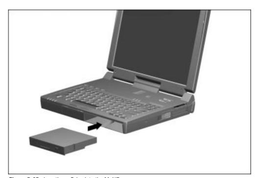
Figure 5-25. Inserting a Drive into the MultiBay
