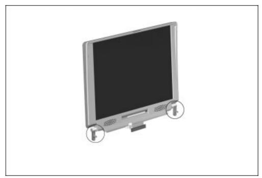
Figure 5-52. Proper Position of the Display Clutches
