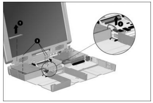
Figure 5-33. Removing the Left Rear Cover and Disconnecting the Power Supply Cable
