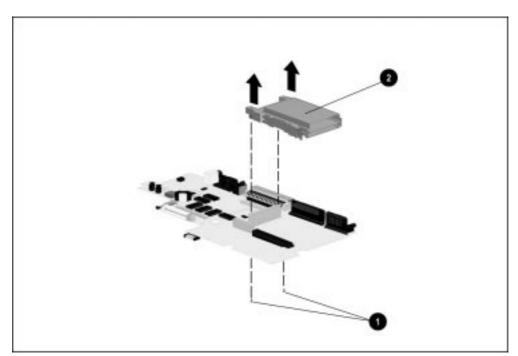
Figure 5-63. Removing the PC Card Assembly
