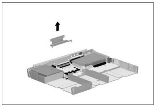
Figure 5-58. Removing the Expansion Connector Shield
