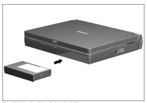
Figure 5-14. Inserting a Battery Pack into the MultiBay
