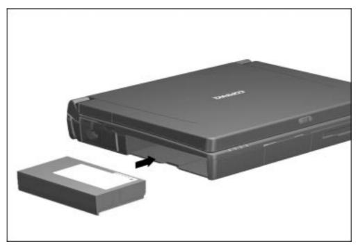
Figure 5-13. Inserting a Battery Pack into the Battery Bay
