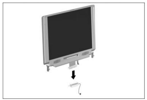
Figure 5-50. Disconnecting the Auxiliary Battery Assembly from the Display Ground Cable
