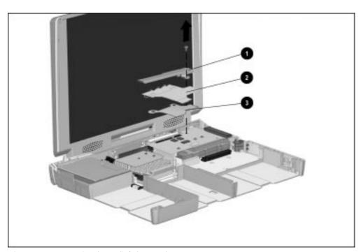
Figure 5-37. Removing the Audio/USB Board
