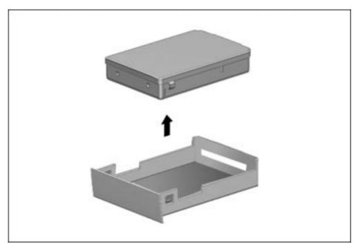
Figure 5-17. Removing the Hard Drive from the Hard Drive Tray
