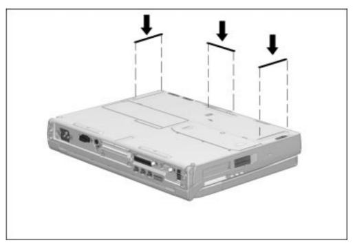
Figure 5-8. Installing the Computer Feet
