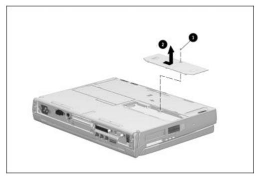
Figure 5-26. Removing the Memory Expansion Slot Cover
