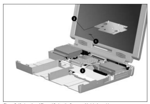
Figure 5-40. Location of Thermal Pad on the Processor Module Assembly
