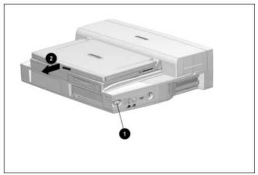
Figure 5-4. Undocking the Computer from the ArmadaStation
