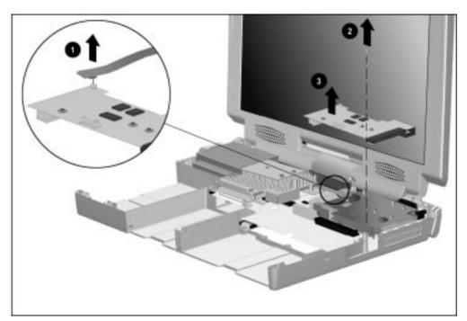
Figure 5-38. Removing the Modem Board
