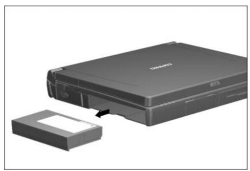
Figure 5-10. Removing a Battery Pack from the Battery Bay
