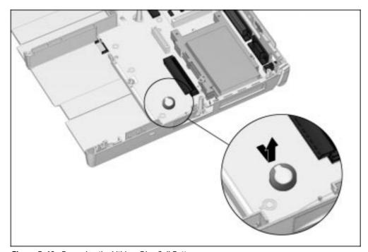
Figure 5-42. Removing the Lithium Disc Cell Battery
