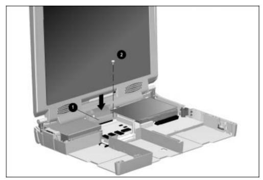
Figure 5-54. Connecting the Display Video Cable
