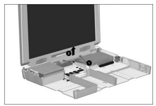
Figure 5-46. Disconnecting the Display Video Cable
