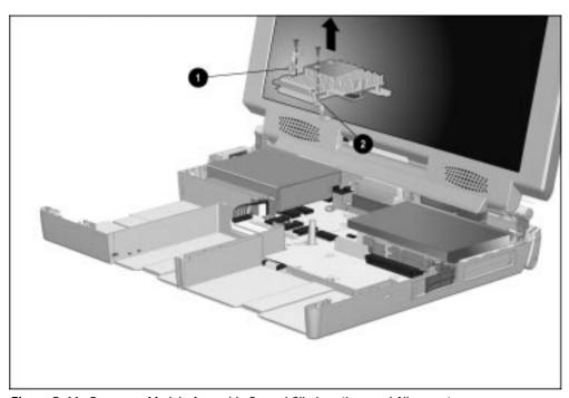
Figure 5-44. Processor Module Assembly Ground Clip Locations and Alignment
