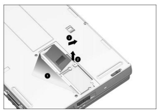
Figure 5-27. Removing a Memory Expansion Board
