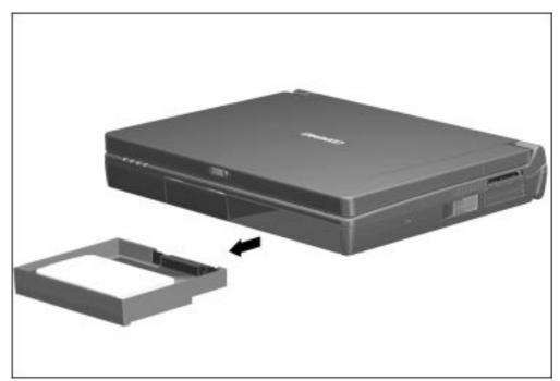
Figure 5-22. Removing the Hard Drive Assembly from the MultiBay
