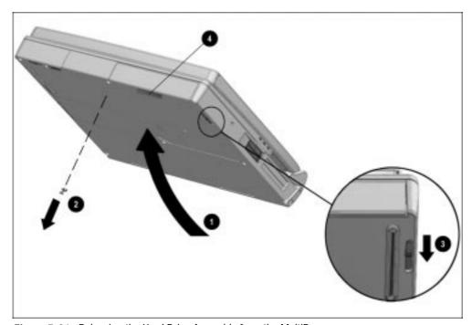
Figure 5-21. Releasing the Hard Drive Assembly from the MultiBay
