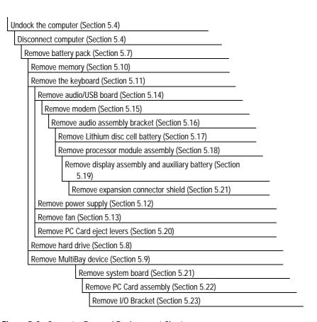
Figure 5-3. Computer Removal Replacement Chart
