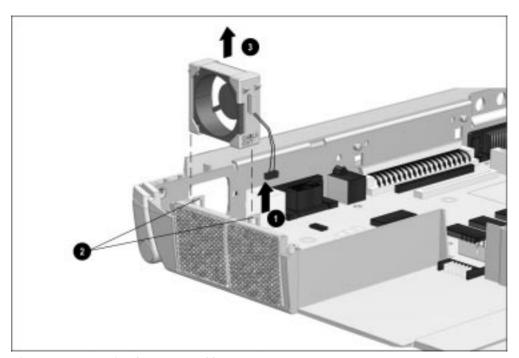
Figure 5-35. Removing the Fan Assembly
