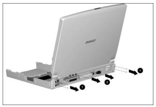
Figure 5-48. Removing the Display Assembly and Auxiliary Battery Assembly Screws
