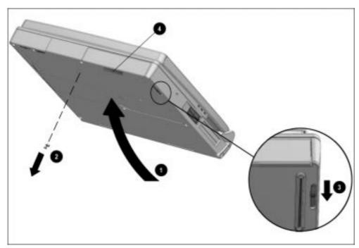
Figure 5-11. Releasing a Battery Pack from the MultiBay
