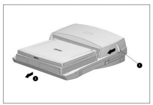
Figure 5-5. Undocking the Computer from the Armada MiniStation
