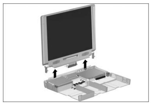
Figure 5-49. Removing the Display Assembly
