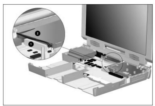
Figure 5-41. Routing the Auxiliary Battery Cable
