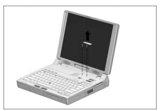
Figure 5-31. Removing the Keyboard Warning Label and Screws
