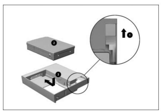
Figure 5-20. Inserting a Hard Drive into a Broadway Hard Drive MultiBay Adapter
