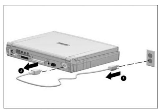
Figure 5-6. Disconnecting the Computer
