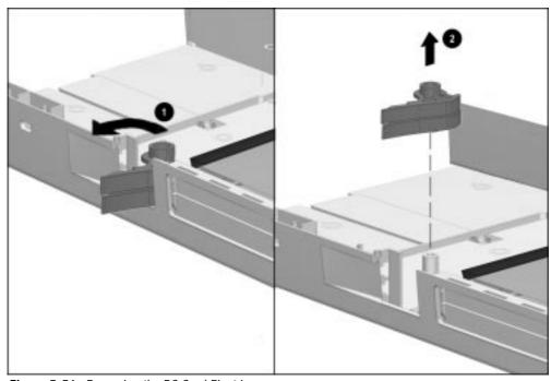
Figure 5-56. Removing the PC Card Eject Levers
