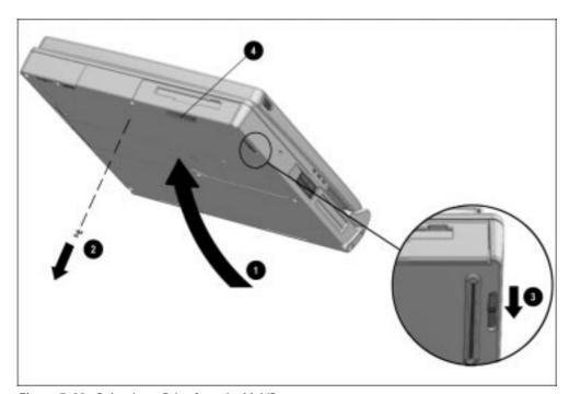
Figure 5-23. Releasing a Drive from the MultiBay
