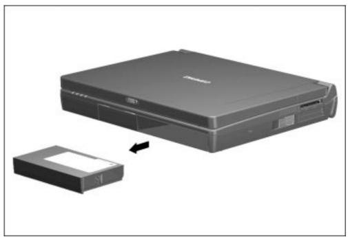
Figure 5-12. Removing a Battery Pack from the MultiBay
