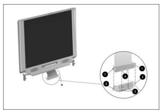
Figure 5-51. Attaching the Display Ground Cable to the Auxiliary Battery Assembly
