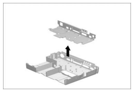
Figure 5-64. Removing the I/O Bracket
