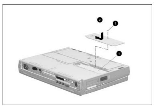
Figure 5-29. Replacing the Memory Expansion Slot Cover
