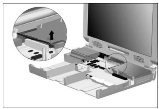
Figure 5-47. Disconnecting the Auxiliary Battery Cable
