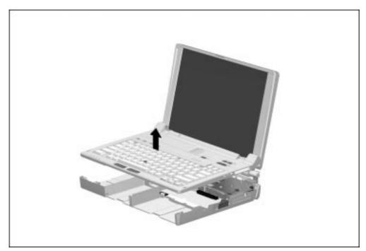
Figure 5-32. Removing the Keyboard Assembly
