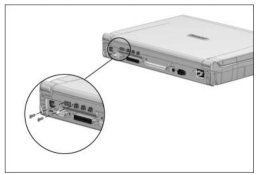
Figure 5-36. Removing the Audio/USB Board Screws
