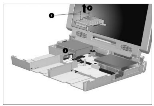
Figure 5-43. Removing the Processor Module Assembly
