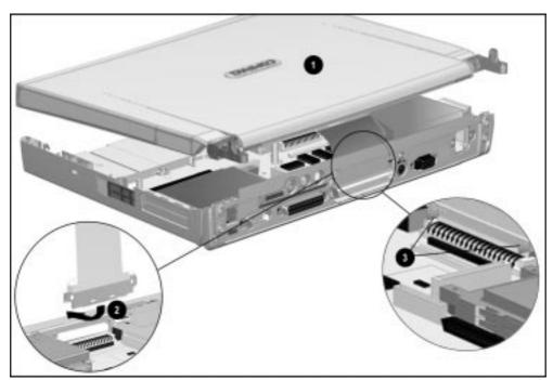
**Figure 5-53.** Attaching the Display Ground Cable/Auxiliary Battery Assembly to the Computer Base Assembly
