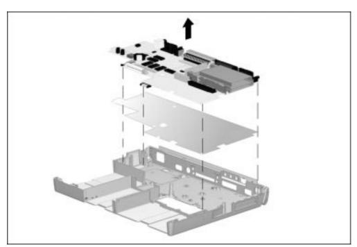
Figure 5-62. Removing the System Board and Insulator
