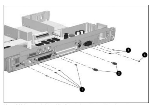
Figure 5-61. Removing the System Board Screwlocks and Keyboard/Mouse Connector Screw
