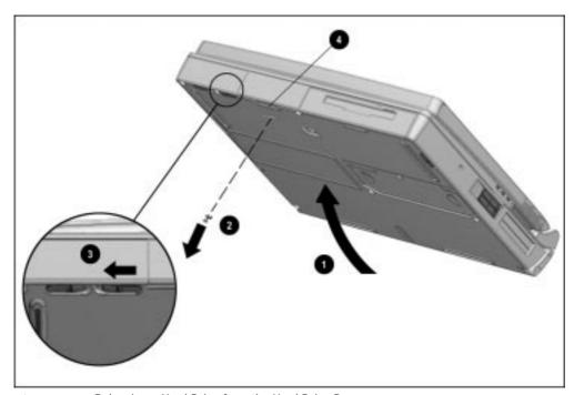
Figure 5-15. Releasing a Hard Drive from the Hard Drive Bay
