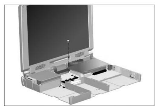
Figure 5-45. Removing the Display Video Cable Connector Screws
