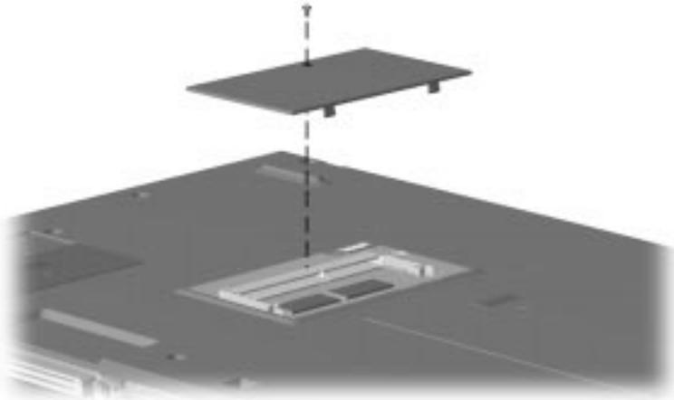
1. Insert the memory expansion board into the empty memory expansion slot at a 45-degree angle. Then slide it gently into place until it is seated while tilted.
