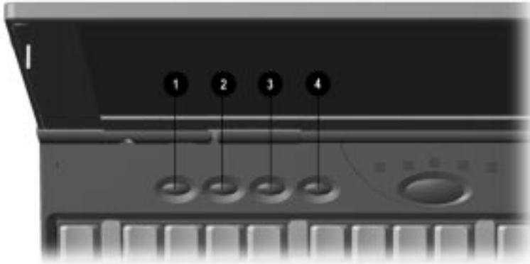
By assigning schemes to the programmable keys, you can create multiple sets of key assignments tailored to your own needs or to accommodate more than one user.
