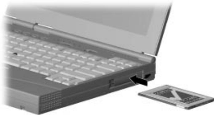
If you are running Windows 95 or later and your computer is on, the computer automatically configures a plug and play card and most other PC Cards. If the computer is turned off or in Suspend, a card is not configured until you turn on the computer or exit Suspend.
