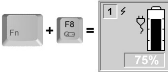
The percentage of battery charge remaining for the battery pack is shown at the bottom of the popup. If the battery pack is charging, a lightning bolt symbol appears to the right of the box. If AC power is connected, the power connector is shown.
