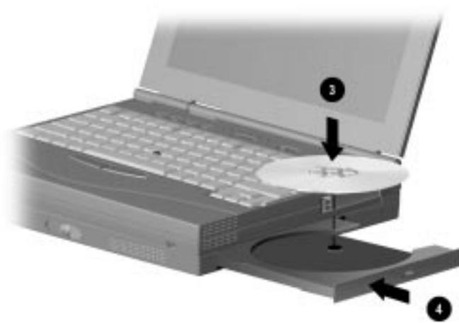
The light on the CD-ROM drive or DVD-ROM drive turns on while the disc is checked and the table of contents is being read. The light turns off when the drive is ready to receive commands.
