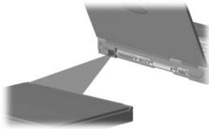
The infrared port produces an invisible beam of infrared light to communicate with another infrared-equipped device.
