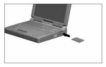
If you are running Windows 95 and your computer is on, the computer automatically configures a Plug and Play card and most other PC Cards. If the computer is turned off or in Suspend, a card is not configured until you turn on the computer or exit Suspend.
