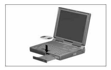
5 Push lightly on the bezel of the CD loading tray to close it.
