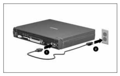
**NOTE:** In Japan, you must first plug the power cord into the 3-to-2prong plug adapter included with the computer. Ensure that the ground wire is connected to a safe earth ground, then plug the 3to-2-prong plug adapter into the electrical outlet.
