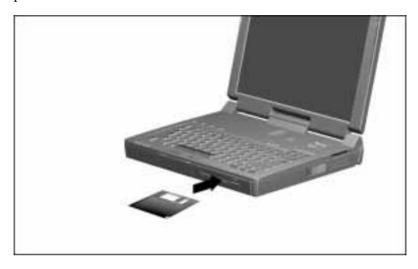
If the diskette is inserted correctly, it drops into position in the diskette drive and the diskette drive button pops out.
