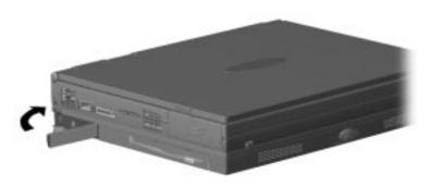
7. Slide display latches forward **0**, to open the computer **2**.
