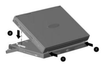
Push in the expansion lever to secure the computer to the M35EÛ.
