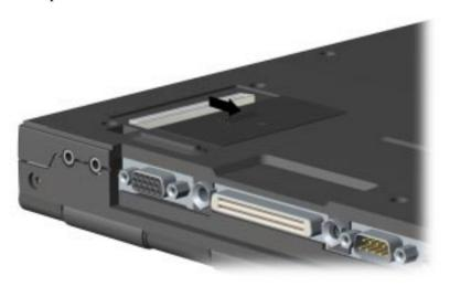
4. On the M35EU, press the expansion lever release button **①**, to release the expansion lever 2.
