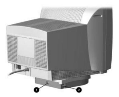
These USB connectors operate as a pass-through system. Your computer must have a USB host controller installed for any USB-connected devices to operate.
