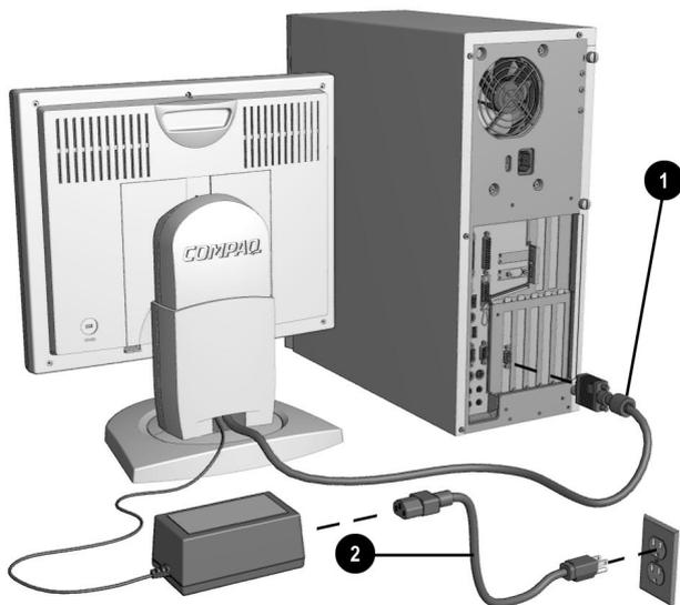
3. Connect one end of the AC power cord ❷ to the AC adapter and the other end to an electrical outlet that is easily accessible and close to the monitor.
