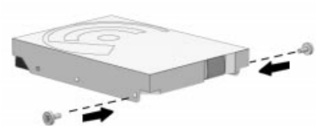
Installing the Flanged Screws into the Hard Drive
