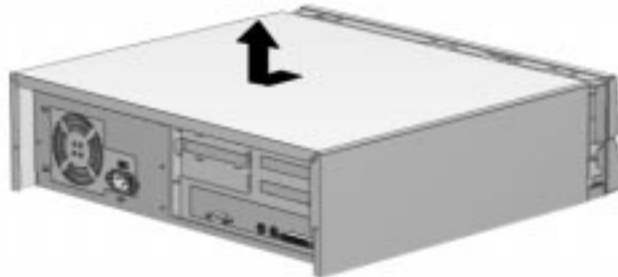
Removing the Desktop Computer Cover
