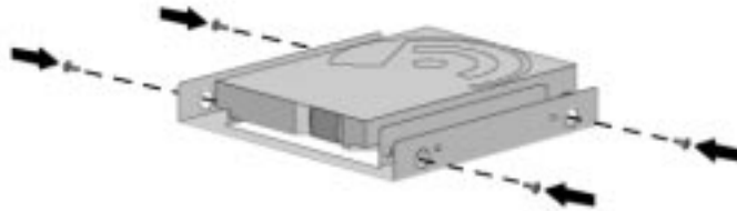
Placing the Hard Drive and Inserting Screws into the Bracket
