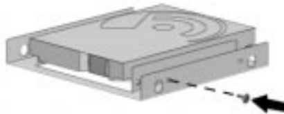
Inserting the Guide Screw into the Bracket
