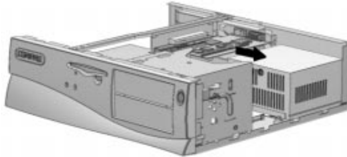
Removing the Graphics Controller Board from the PCI Expansion Slot
