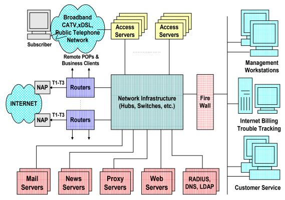
Figure 2. Architectural Overview of an Internet Service Provider
