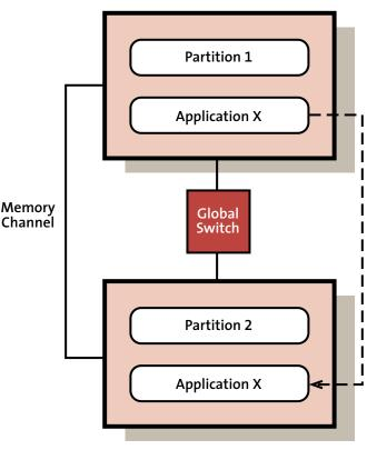
This *TruCluster* Server is operating within a single system and provides high availability via automated partition failover. In this scenario, partition 2 takes over the application running on partition 1 automatically and transparent to end-users
