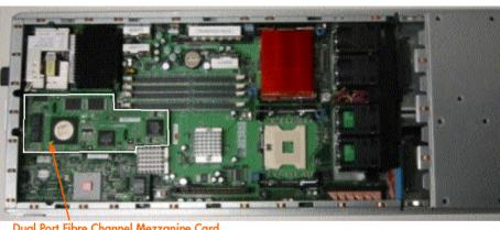
Figure 5. Dual Port Fibre Channel Mezzanine Card for ProLiant BL20p G2 SAN connectivity
