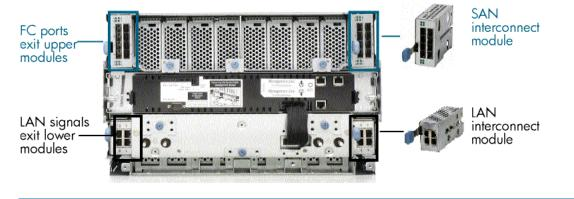
Figure 10. Rear of server blade enclosure with both SAN and LAN interconnect modules installed
