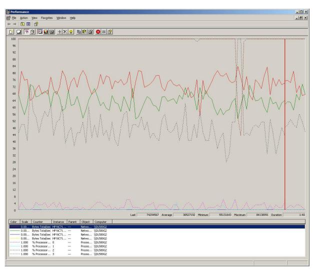
Two solid lines (red and green) indicate that the network load balancing has used two NICs running at around about 65% and 75% loading each. Processor 2 in the DL580 server is running at 90–100% since this is receiving data from the 2-way ML370 G4 server.
