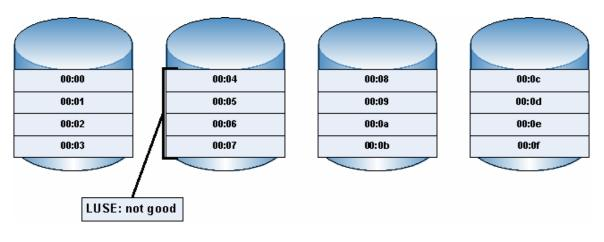
In Figure 7, the LDEV numbering allows the LUSE to be spread across the four array groups shown.
