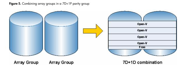
The two array groups, paired in this way, must be connected to two separate ACPs. HP has successfully used this mode in Exchange deployments, and is it recommended, even though it uses a RAID 5 distributed parity redundancy scheme.
