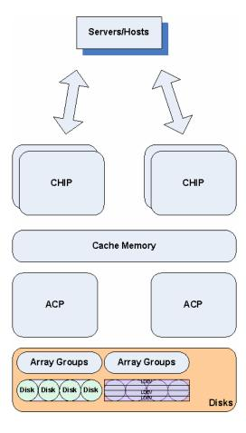
Channel Host Interface Processors (CHIPs) control data movement between the host servers and cache memory. CHIPs come in pairs for redundancy. There are different types, depending on the host interconnect mode chosen (such as Fibre Channel, ESCON, and FICON). CHIPs are the interface to the host bus adapter (HBA), with intermediate fabric components, depending on the topology and protocol chosen.
