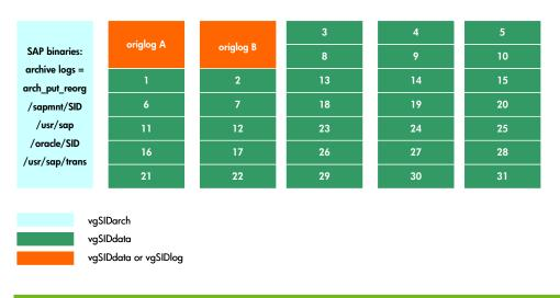
Figure 12. Sample storage layout for SAP with HP-UX on an XP disk array
