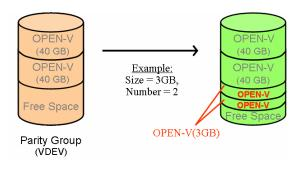
The goal is to have a reasonable number of LUNs available on the operating system level maintaining the balance with the fewest possible LUNs to minimize the administrative overhead and distribute the I/O load effectively over all components in the I/O path from the Fibre Channel Adapter (FCA) down to the disks.
