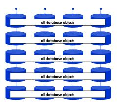
Figure 3 illustrates that all database objects of an SAP instance are evenly distributed across all available disks and controllers, with large logical volumes striped across multiple disks.
