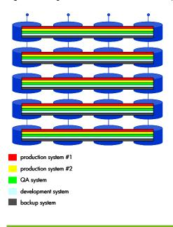
To prevent hotspots following hardware upgrades (after the new data is stored on newly added disks), the disk array should be equipped with the reasonable number of disks during initial installation.
