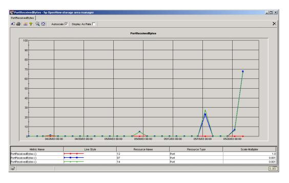
**Figure 5.** Text-based query across all Fibre Channel switches in the domain, using a characteristic throughput metric—Device Received Bytes—as a measure to compare all four switches and identify potential hot spots.
