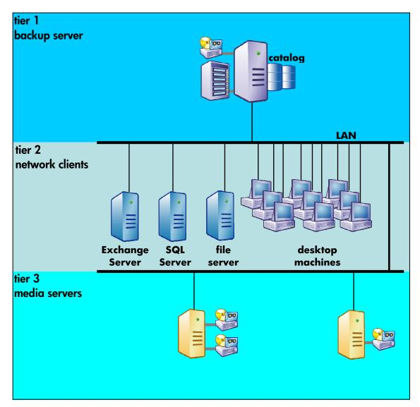
Figure 1. Data Protector Express has a three-tier architecture for performance, reliability, and flexibility
