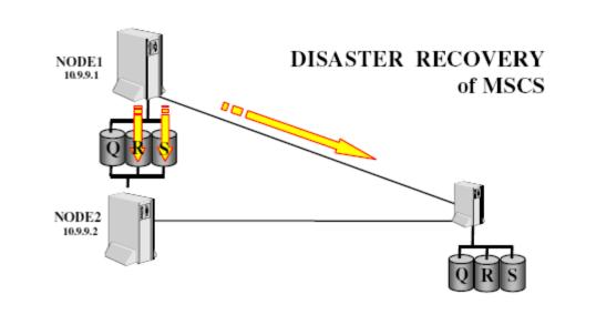
The target platform can be located anywhere in the world and brought back online to stand in for a failed production Exchange instance.
