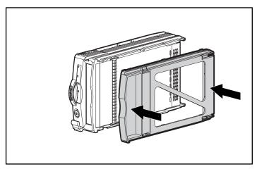
Figure 6. Installing the tape drive height converter
