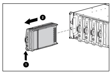
Figure 5. Removing a drive
