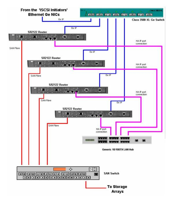
Figure 42: Maximum SR2122 Cluster Configuration Using HA Ports
