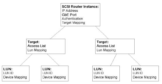
Figure 12: SCSI Router Instance Structure
