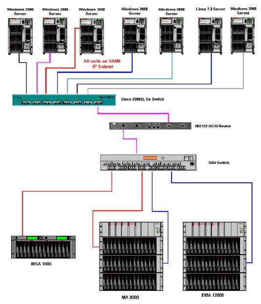
Figure 40: Example of Multiple OS Systems in a Non-Redundant Path Configuration
