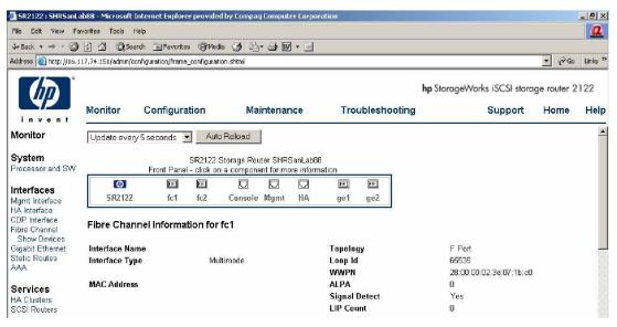
Figure 2: GUI Display of the FC port WWPN
