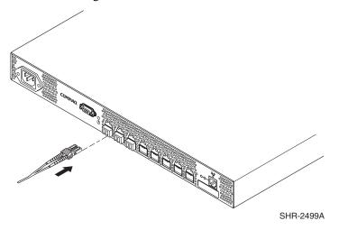
Figure 2–8: Installing an SFP
