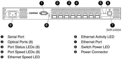
Figure 1–1: SAN Switch 2/8 EL front panel
