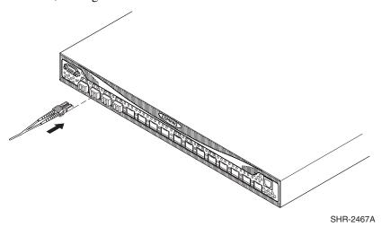
Figure 2-11: Installing an SFP
