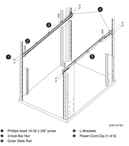
Figure 2-6: Attaching the Outer Slide Rails to the 9000 Series Rack
