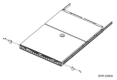
Figure 2-5: Attaching the Rear Rack Mount Brackets
