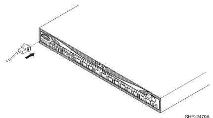
2. Connect the Serial cable to the SAN Switch 2/16 EL Serial port, see Figure 2–9.
