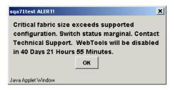
Figure 2-1: Four Switch Limitation Web Tools Error Message
