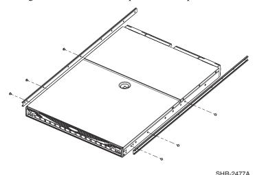
3. Tighten the screws and torque to 15-inch pounds.
