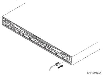
Figure 2-10: Connecting the Ethernet Cable
