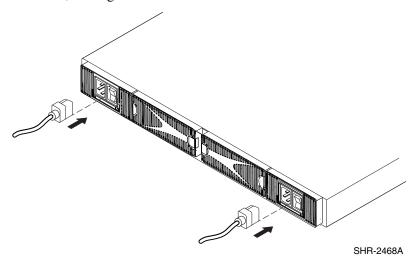
Figure 2-8: Connecting the power cords
