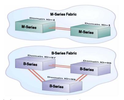
Figure 2: Example of Unique Domain IDs (M-Series Changed to Domains 4 & 5)
