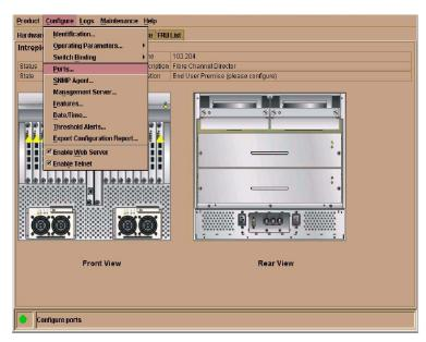
Figure 26: HAFM: Selecting Configure Ports
