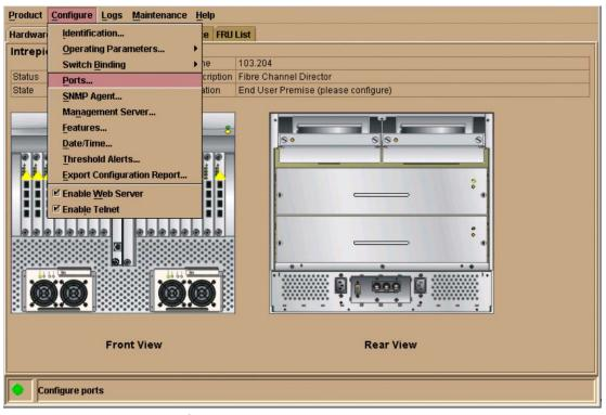
Figure 30: HAFM: Select Configure > Ports
