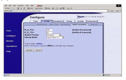
Figure 15: EWS: Selecting Fabric Parameters Tab
