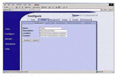
Figure 14: EWS: Selecting Switch Tab
