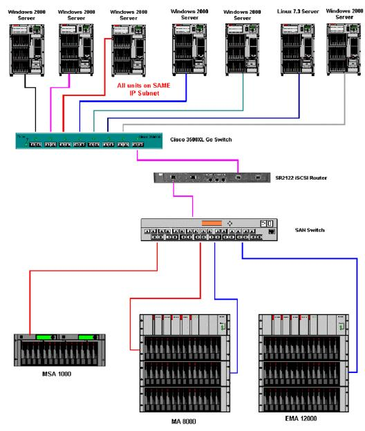
Figure 49: Example of Multiple OS Systems in a Non-Redundant Path Configuration
