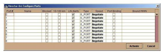
Figure 44: HAFM Configure Ports for 10-100 km setting
