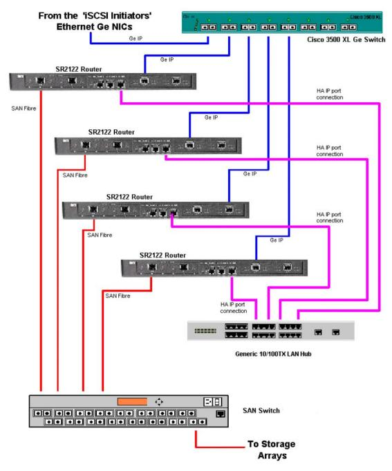
Figure 52: Maximum SR2122 Cluster Configuration Using HA Ports
