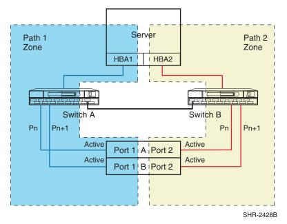
Figure 40: Straight-Cable High Availability Single Fabric Zoned Configuration
