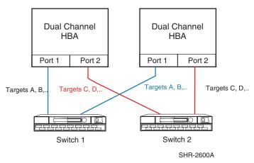
Figure 43: Two PCI Slots with Dual Channel HBAs - NSPOF
