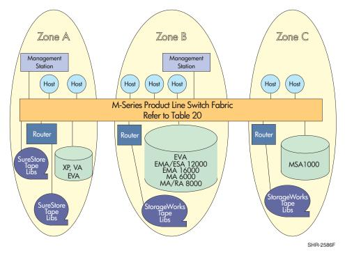
Figure 24: HP StorageWorks SAN using M-Series Switches
