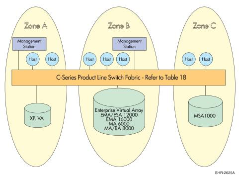
Figure 25: HP StorageWorks SAN using C-Series Switches
