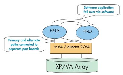
Figure 30: Software application fail-over
