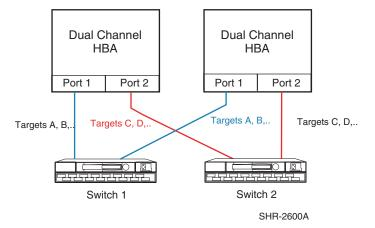
Figure 44: Two PCI Slots with Dual Channel HBAs - NSPOF
