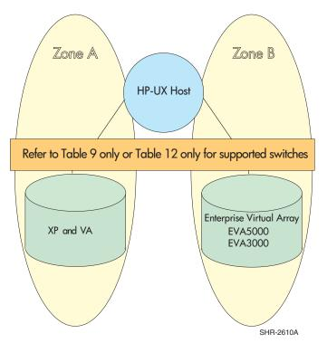
Figure 27: HP StorageWorks SAN with an HP-UX host accessing XP/VA storage in one zone and EVA storage in another zone
