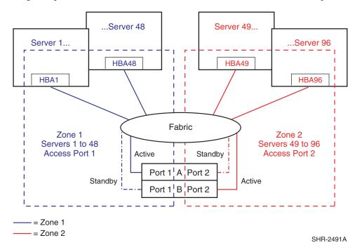
Figure 35: Maximum server example for Tru64 UNIX 5.x with transparent failover using 96 connections and one path per server
