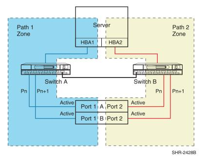
Figure 41: Straight-Cable High Availability Single Fabric Zoned Configuration
