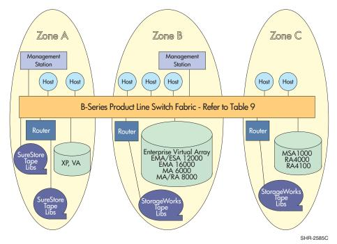
Figure 25: HP StorageWorks SAN using B-Series Switches
