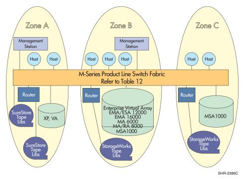
Figure 26: HP StorageWorks SAN using M-Series Switches
