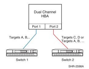
Figure 43: Single PCI Slot with Dual Channel HBA and Two Switches
