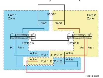
Figure 43: Cross-Cable High Availability Single Fabric Zoned Configuration
