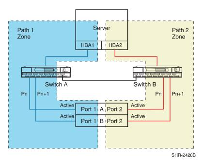
Figure 44: Straight-Cable High Availability Single Fabric Zoned Configuration
