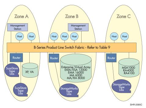
Figure 26: HP StorageWorks SAN using B-Series Switches
