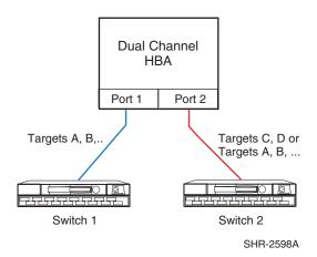
Figure 46: Single PCI Slot with Dual Channel HBA and Two Switches
