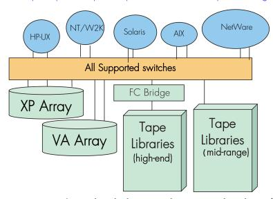
Figure 35: XP/VA with multiple OS's and tapes on a shared SAN fabric, fabric only<sup>1</sup>
