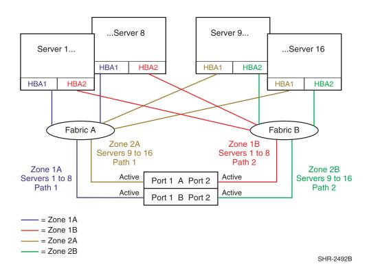
Figure 39: Maximum server example for Windows NT using 16 servers with multiple-bus failover and two paths per server
