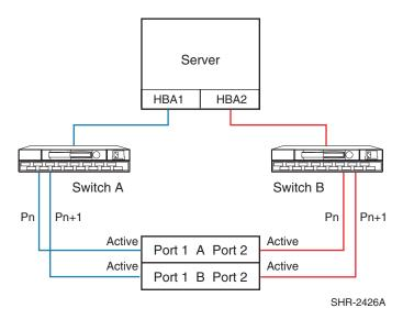
Figure 42: Straight-Cable High Availability NSPOF Configuration
