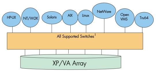
Figure 34: XP/VA with multiple OS's on a shared SAN fabric<sup>1</sup>
