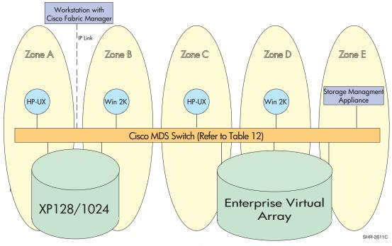
Figure 29: HP StorageWorks SAN using XP 128/1024 and EVA storage with Cisco switch
