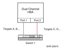
Figure 45: Single PCI Slot with Dual Channel HBA and One Switch
