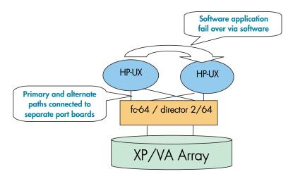
Figure 33: Software application fail-over
