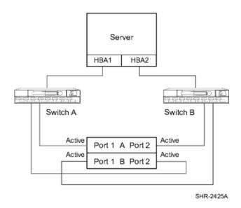
Figure 41: Cross-Cable High Availability NSPOF Configuration
