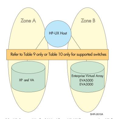
Figure 28: HP StorageWorks SAN with an HP-UX host accessing XP/VA storage in one zone and EVA storage in another zone
