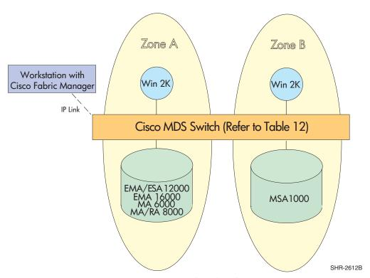
Figure 30: HP StorageWorks SAN using EMA/ESA/MA/RA and MSA Storage with Cisco switch
