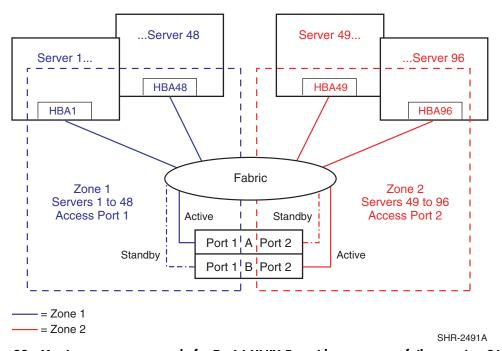
Figure 38: Maximum server example for Tru64 UNIX 5.x with transparent failover using 96 connections and one path per server
