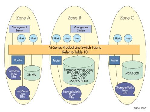
Figure 27: HP StorageWorks SAN using M-Series Switches
