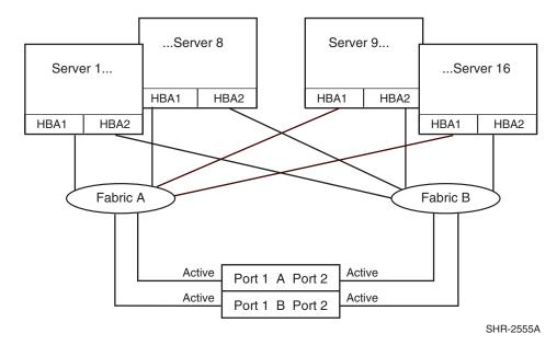
Figure 40: Maximum server example for Windows 2000 using 16 servers with multiple-bus failover and four paths per server
