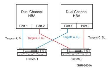
Figure 47: Two PCI Slots with Dual Channel HBAs - NSPOF
