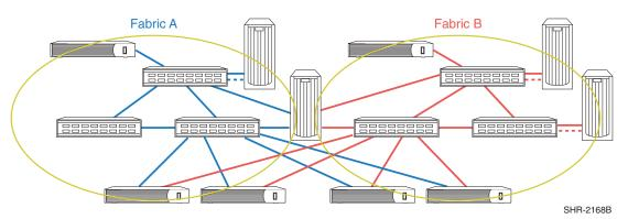
Figure 20: Level 4: Dual Fabric High Availability Multi-Pathing Fault Tolerant
