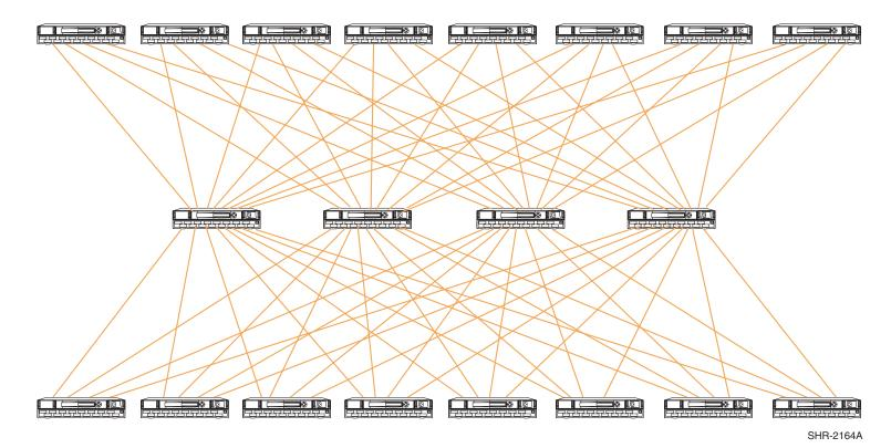
Figure 8: Backbone SAN with 20 Switches
