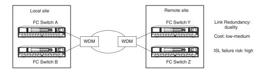
Figure 6: Redundant WDM loop configuration using two (or more) long-haul fiber links
