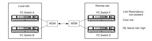
Figure 5: Simple point-to-point configuration using one long-haul fiber link
