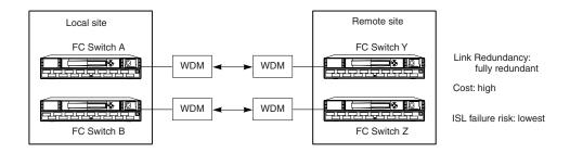
Figure 7: Fully Redundant WDM loop configuration using two (or more) long-haul fiber links
