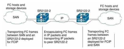
Figure 38: Encapsulating Fibre Channel Frames in IP Packets
