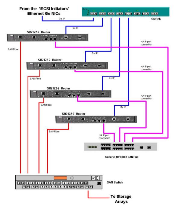
Figure 52: Maximum SR2122-2 Cluster Configuration Using HA Ports
