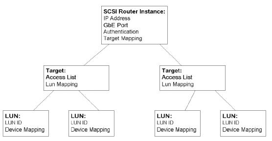
Figure 12: SCSI Router Instance Structure
