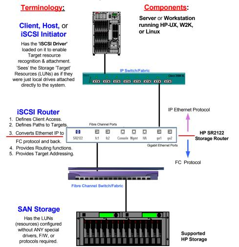
Figure 1: IP/Fibre Channel Network Example
