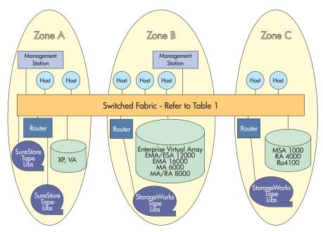
Figure 1: hp StorageWorks SAN using hp StorageWorks core switches and SAN switches with server and storage components from HP and Compaq
