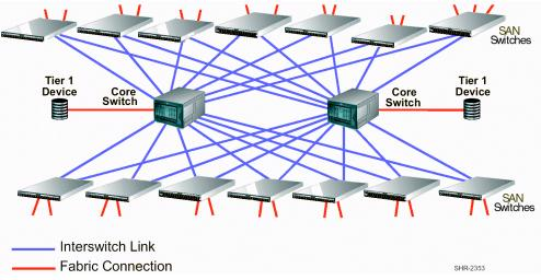
Figure 4: Core switch plus SAN switch hp StorageWorks SAN (2x14 version)
