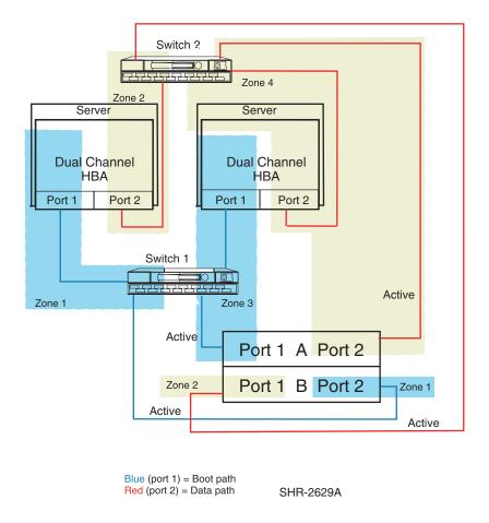
Figure 12: Clustered servers-two dual channel HBAs, two switch cross-cable HA configuration
