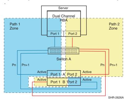
Figure 8: Single server-one dual channel HBA, one switch cross-cable storage configuration
