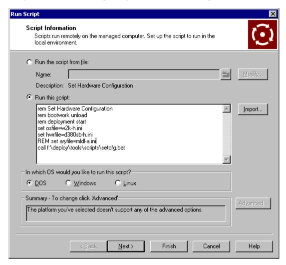
Figure 15: Run Script - Set Hardware Configuration task modified for boot from SAN Deployment
