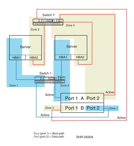
Figure 5: Clustered servers-four single channel HBAs, two switch straight-cable HA storage configuration
