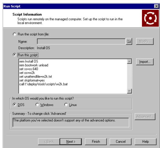
Figure 17 shows a completed **Run Script – Install OS** task.
