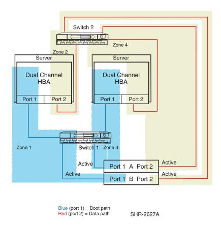
Figure 11: Clustered servers-two dual channel HBAs, two switch straight-cable HA configuration
