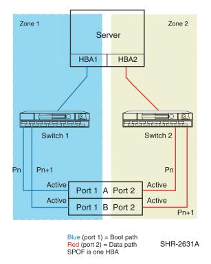
Figure 3: Single server-two single channel HBAs, two switch straight-cable HA storage configuration
