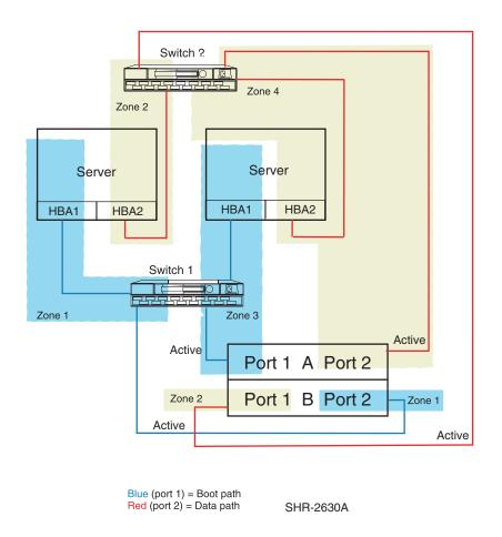
Figure 6: Clustered servers-four single channel HBAs, two switch cross-cable HA storage configuration
