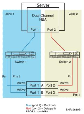
Figure 9: Single server-one dual channel HBA, two switch straight-cable HA storage configuration
