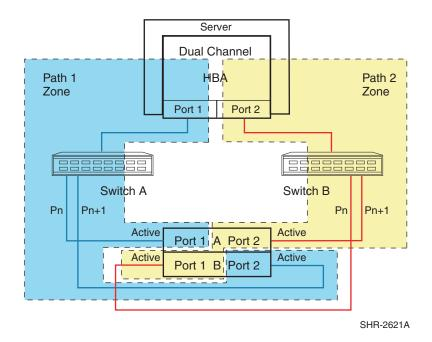
Figure 10: Single server-one dual channel HBA, two switch cross-cable HA storage configuration
