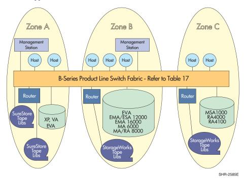
Figure 23: HP StorageWorks SAN using B-Series Switches
