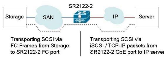
In this example FC storage connects to the Fibre Channel interface of the SR2122-2 Storage Router deployed for iSCSI. The SR2122-2 connects to the IP network through one of its Gigabit Ethernet interfaces. The server accesses the storage served from the router through the IP network.
