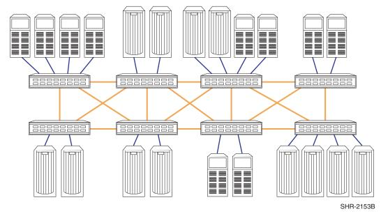
Figure 4: Modified Meshed Fabric SAN
