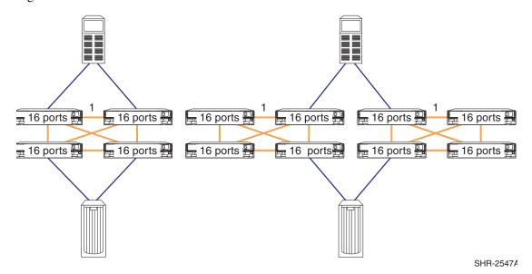
up to 52 ports for server and storage connectivity. Implementing the same topology using two fabrics provides up to 104 ports for server and storage connectivity. This is shown in Figure 19.
