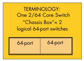
Figure 21: Core Switch definition
