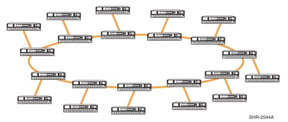
Figure 6: Ring Fabric SAN with Satellite Switches
