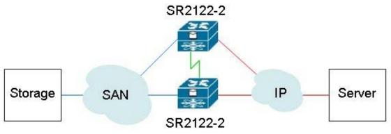
In this example configuration, two storage routers are connected (clustered) together to allow the storage routers to back each other up in case of failure.
