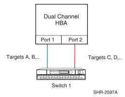
Figure 41: Single PCI Slot with Dual Channel HBA and One Switch
