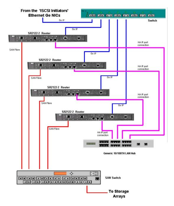
Figure 54: Maximum SR2122-2 Cluster Configuration Using HA Ports
