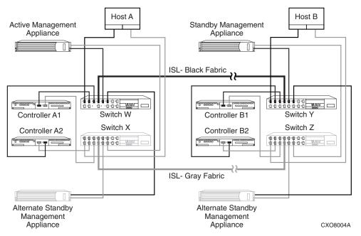
Figure 44: Continuous Access EVA basic configuration
