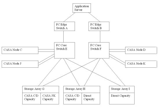
Figure 62: Multiples CASA Supporting Mix of Arrays
