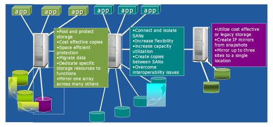
Figure 59: Cascaded CASA Configuration with Three Sites
