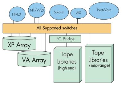
Figure 31: XP/VA with multiple OS's and tapes on a shared SAN fabric, fabric only<sup>1</sup>
