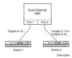
Figure 42: Single PCI Slot with Dual Channel HBA and Two Switches
