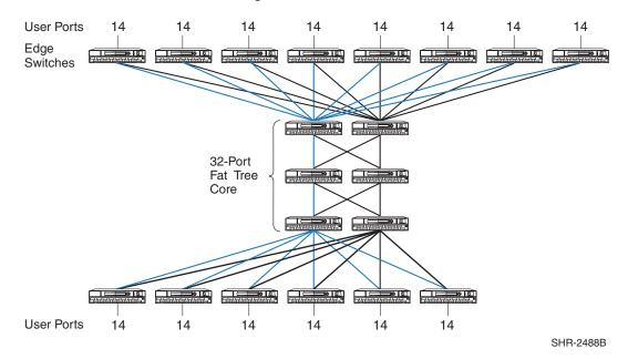
Figure 63: Example of Core Switch Plus Edge Switch Configuration
