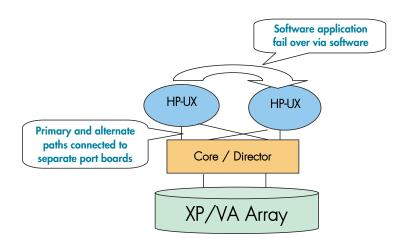
Figure 29: Software application fail-over
