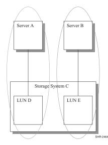
Figure 56: Multiple Security Domains on One Storage System
