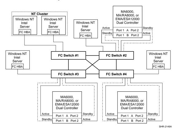
Figure 7. Four Switches, Meshed Fabric Configuration Example
