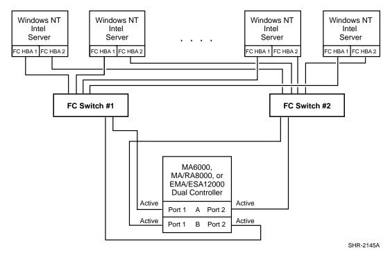
Figure 3. Two Switch HA Fabric Configuration Example
