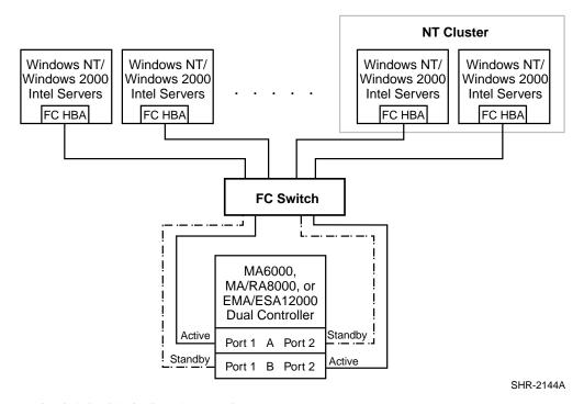
Figure 2. One Switch Fabric Configuration Example
