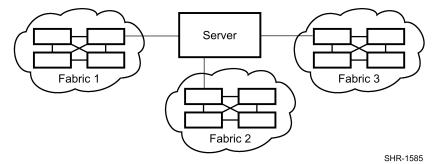
Figure 1. One Server to Multiple 4-Switch Fabrics
