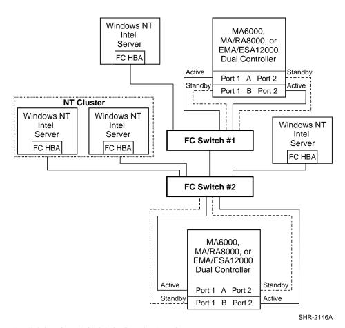
Figure 4. Two Switches, Cascaded Fabric Configuration Example
