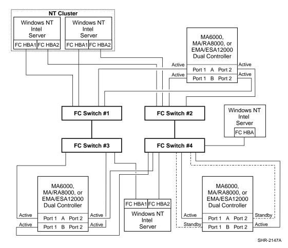
Figure 5. Four Switches, Cascaded HA Fault Tolerant Fabric Configuration Example
