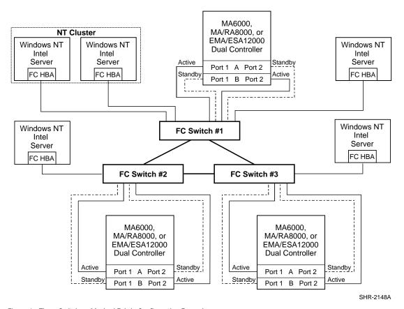
Figure 6. Three Switches, Meshed Fabric Configuration Example
