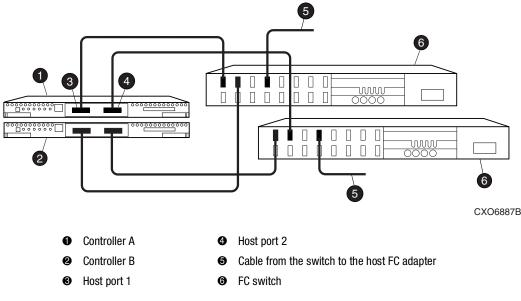
Figure 5–3. Controller pair failover cabling
