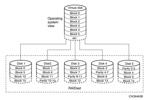
Figure 2–14. A 5-member RAIDset using parity
