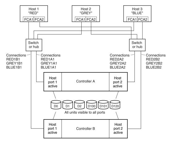
NOTE: FCA = Fibre Channel Adapter
