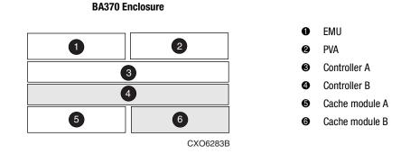
Figure 1–2. Location of controllers and cache modules in a BA370 enclosure
