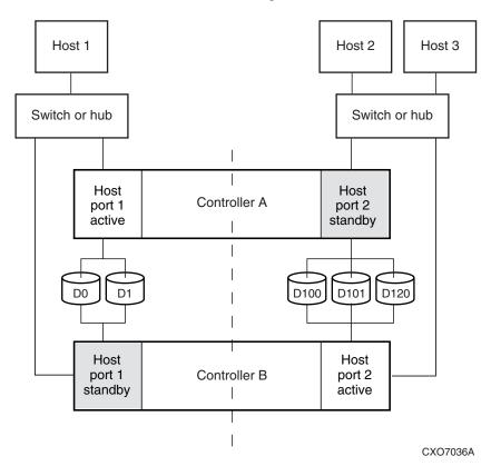
Figure 1-5. Transparent failover-normal operation
