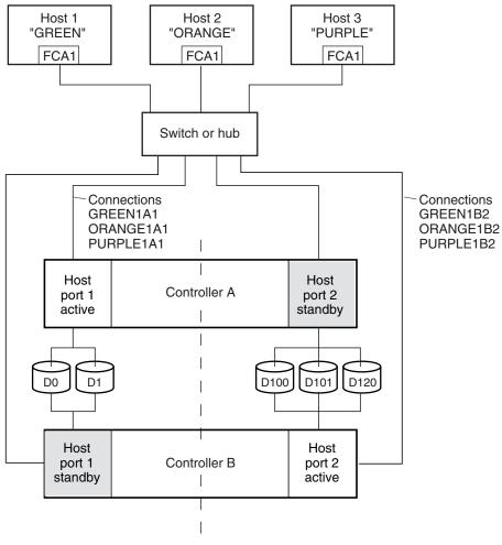
NOTE: FCA = Fibre Channel Adapter
