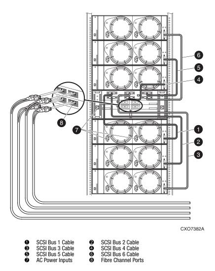
Figure 3–2. Single-Bus Enterprise Storage RAID Array Storage System
