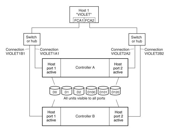
NOTE: FCA = Fibre Channel Adapter
