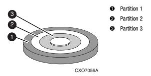
Figure 2–17. One example of a partitioned single-disk unit
