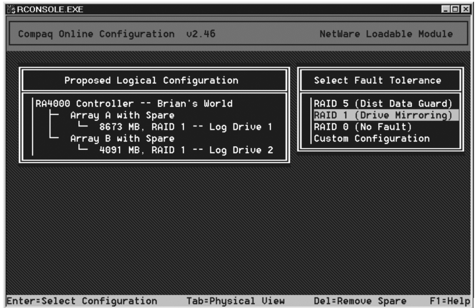
Figure 5-29. Auto-configuration wizard with RAID 1 fault tolerance selected
