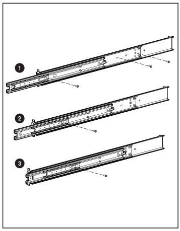
Figure 4-10. Attaching the sliding bracket rails to the rack mounting brackets
