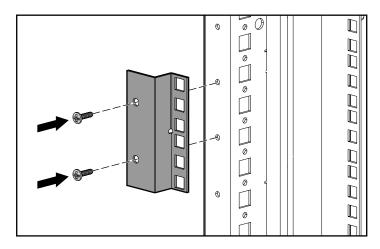
Secure the inner mounting rail to the adapter with a 10-32 nutbar:
