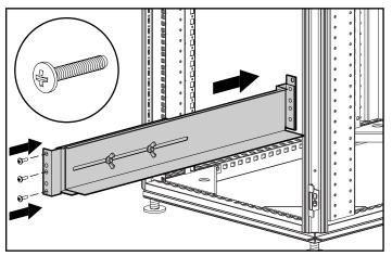
Figure 4-4. Fastening the fixed rail to the front of the rack
