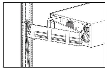
Figure 4-19. Routing the cables
