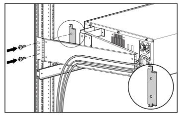
Figure 4-18. Attaching the cable management arm to the rack
