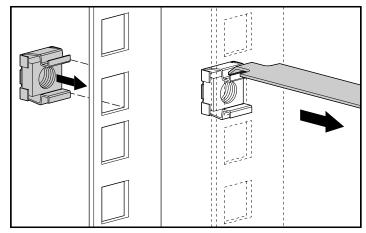
Figure 4-2. Inserting cage nuts
