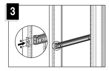
Attach the Latch Bracket to each mounting bracket with the latch receptacle facing the front of the rack.
