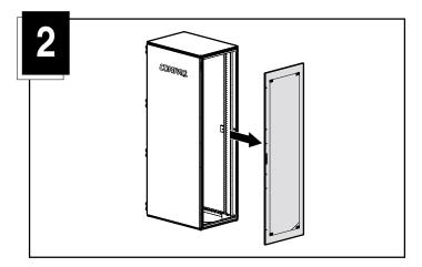
**NOTE:** If a short rear door was removed, an additional hinge must be added to the rear of the rack before installing the extension, proceed to step 3B.
