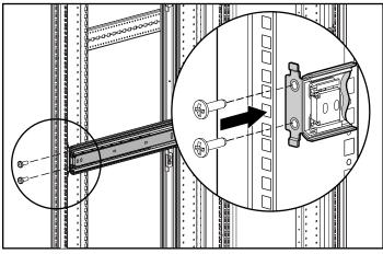
Figure 4-11. Attaching the front of the rack mounting bracket assembly
