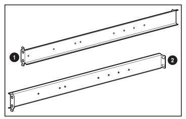
Figure 4-8. Orienting the rack mounting brackets
