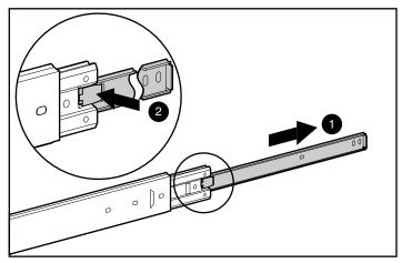
Figure 4-7. Removing the component rail
