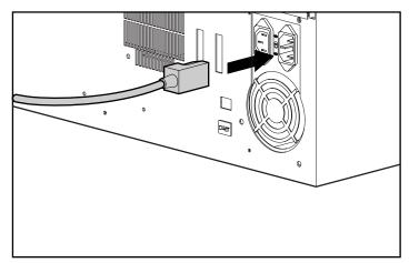
Figure 4-17. Attaching the AC power cord
