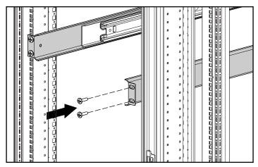
Figure 4-12. Attaching the back of the rack mounting bracket assembly
