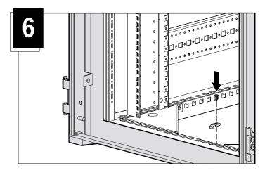
Attach a grounding strap from the ① grounding stud on the lower left side of the door extension to the ② system chassis rail.
