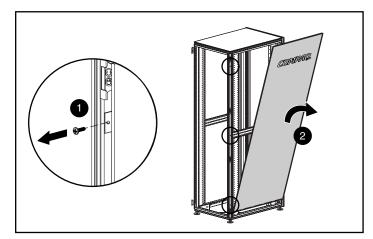
Figure 3-4. Removing a sidewall panel
