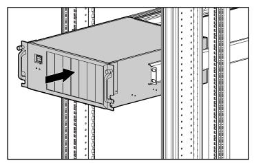
Figure 4-15. Inserting the unit into the rack
