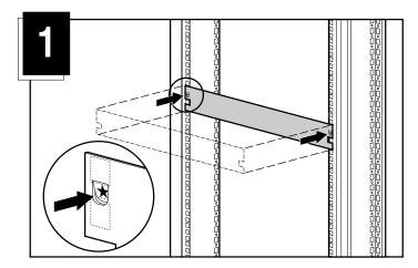
• Insert cage nuts on the rear of the rack in each of the holes marked using the template.
