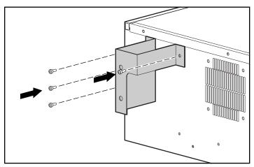
Figure 4-14. Attaching the cable management arm bracket to the unit
