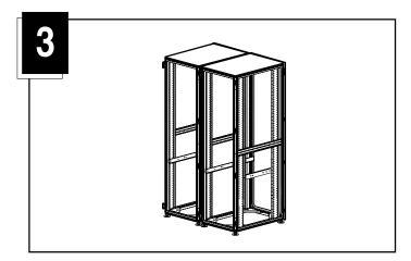
Use either a 24-inch bracket or a 600-mm bracket, depending on the floor layout. Attach three brackets to the front and three brackets to the rear of each rack set, using two T30 screws in each bracket.
