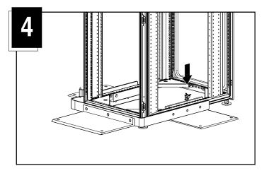
Tighten the front stabilizer foot screws. Reinstall any rack components.
