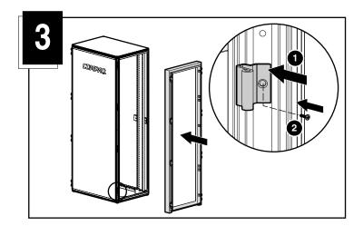
**1** Install one screw fastener in the top right of the rack frame.
