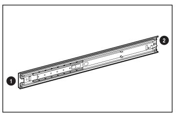
Figure 4-9. Orienting the sliding bracket rails
