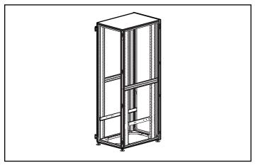
Figure 4-6. Rack ready for component installation
