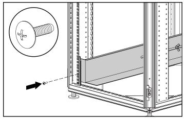
Figure 4-5. Fastening the fixed rail to the back of the rack
