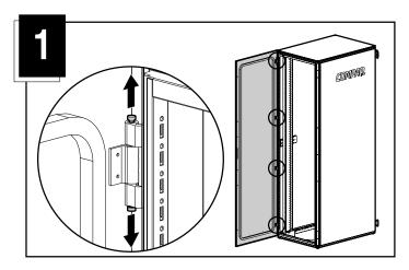
Lift the door away from the rack. Place the door in an upright position, taking care to protect from damage.
