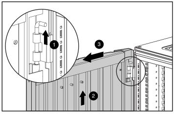
Figure 3-3. Removing a door
