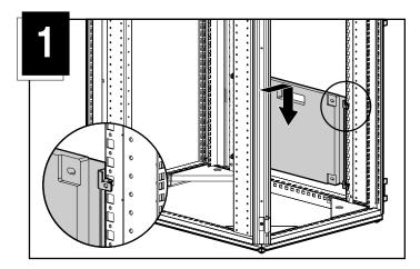
Insert four 5.5-mm, self-tapping screws and tighten.
