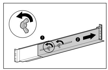
Figure 4-3. Adjusting the fixed rails
