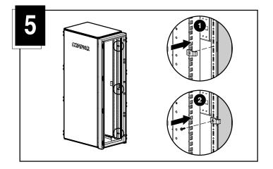
Install one screw fastener and one T-25 5.5-mm torx head screw in the bottom right of the rack frame.
