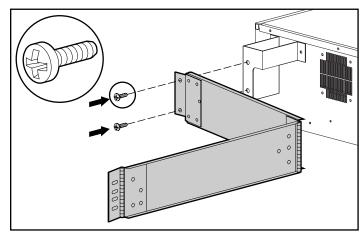
Figure 4-16. Attaching the cable management arm to the bracket
