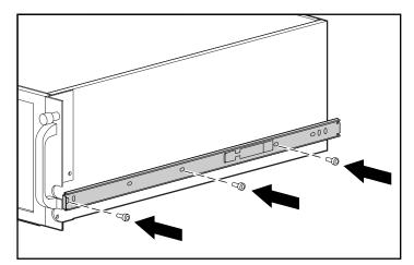
Figure 4-13. Attaching the component rails to the chassis
