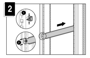
Align the rail with the holes on the front of the rack. Insert two M6 screws and begin to tighten. Insert a rail cover base, then extend the rail and press it against the rack to help properly align the screws, then tighten.
