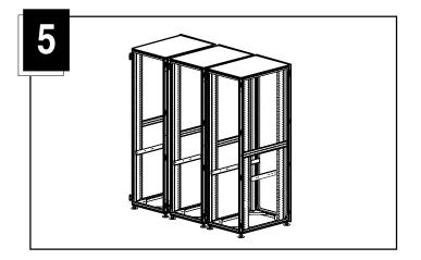
Attach a side panel to each end, and reattach the front and rear doors.
