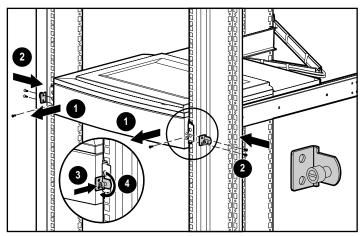
Figure 2-24. Attaching the stabilizing bracket
