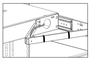
Figure 2-10. Attaching the cables to the cable management arm
