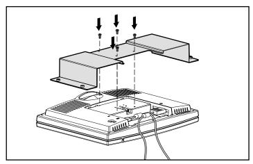
Figure 2-19. Attaching the fixed mounting bracket
