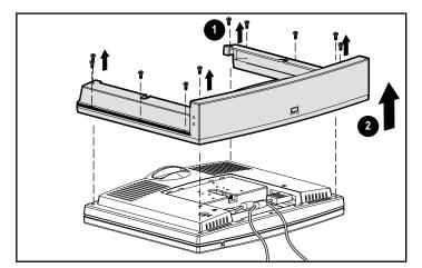
Figure 2-17. Removing the plastic frame
