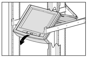
Figure 2-13. Setting the monitor viewing angle
