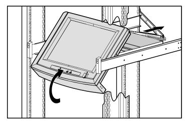
Figure 2-11. Using the retractable tray
