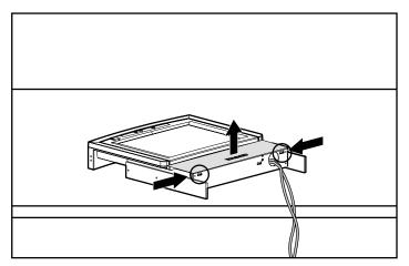
Figure 2-5. Removing the tray cover
