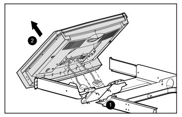
Figure 2-16. Removing the monitor from the tray
