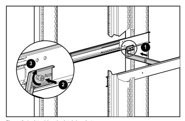
Figure 2-4. Attaching the latch bracket
