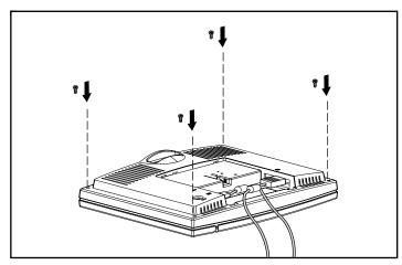
Figure 2-18. Inserting the monitor case screws
