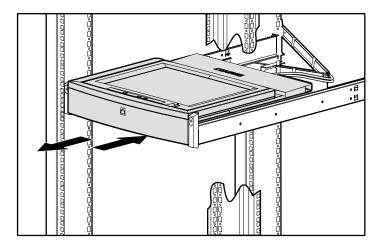
Figure 2-12. Accessing the monitor
