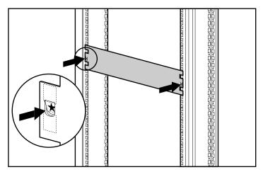
Figure 2-1. Measuring with the 2U template
