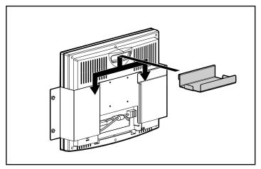
Figure 2-20. Placing the power supply tray
