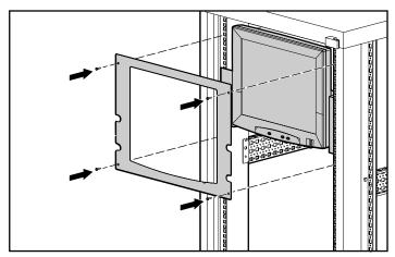
Figure 2-23. Attaching the faceplate
