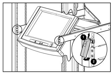
Figure 2-7. Attaching the retma rail covers
