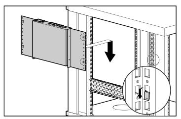
Figure 2-2. Mounting the 2-Port unit to the side of the rack
