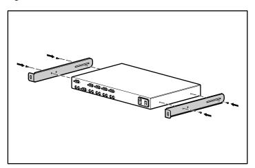
Figure 2-12. Attaching the slide rail brackets
