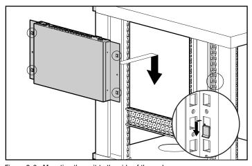
Figure 2-6. Mounting the unit to the side of the rack
