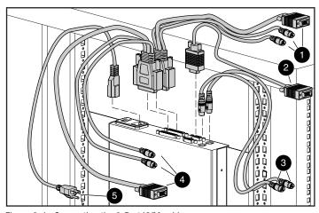
Figure 2-4. Connecting the 2-Port KVM cable
