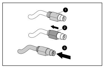
Figure 3-1. Disconnecting the keyboard or mouse cable
