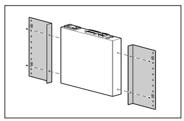
Figure 2-1. Attaching the 2-Port side-mount rails
