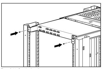
Figure 2-11. Securing the rails
