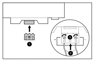
Figure 3-8. Connecting the wires
