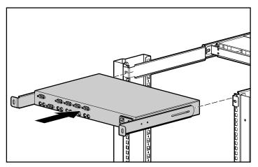
Figure 2-10. Sliding the switch box into the rack
