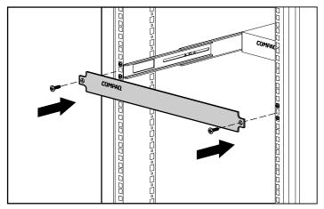
Figure 2-19. Securing the front cover panel
