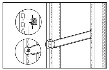
Figure 2-15. Inserting a cage nut
