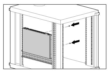
3. Use a screw on each side to secure the side-mounted unit to the rack.
