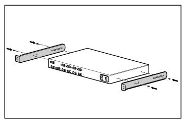
Figure 2-8. Attaching the slide rail brackets
