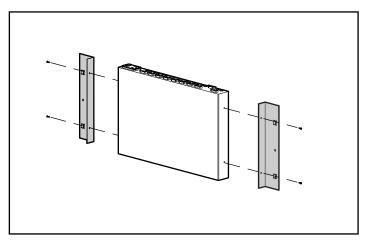
Figure 2-5. Attaching the side-mount rails
