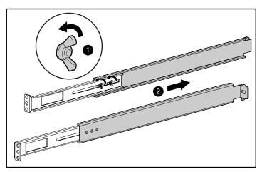
Figure 2-14. Adjusting the length of a rack-mounting bracket
