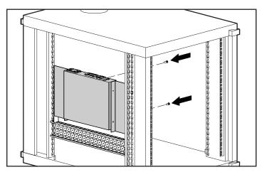
Figure 2-3. Securing the 2-Port side-mount installation
