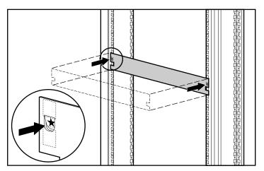
Figure 2-13. Measuring with the template
