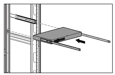
Figure 2-4: Installing the router into the rack
