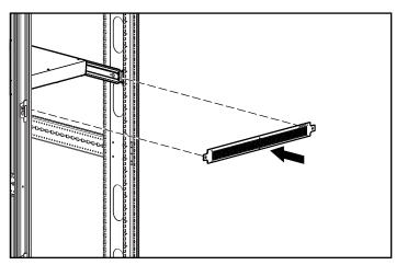
Figure 2-5: Attaching the bezel to the rack
