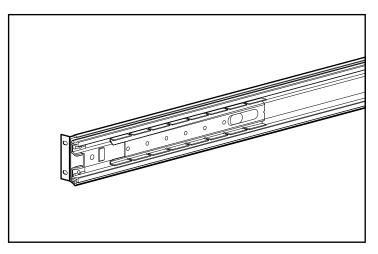
3. Slide the rail out until an opening appears, allowing you to insert the screws.
