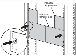
Use the template shipped with the library to mark the location of the mounting hardware on the mounting rails of the storage cabinet.
