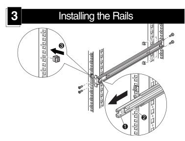
e. Remove the template, then attach the rails using the supplied fasteners. Rail front brackets are threaded to directly accept screws. Rear brackets are not threaded and require installation of cage nuts in the storage cabinet's rear vertical rails. Refer to the *Compaq Rack Products Reference Guide* for detailed cage nut installation instructions.
